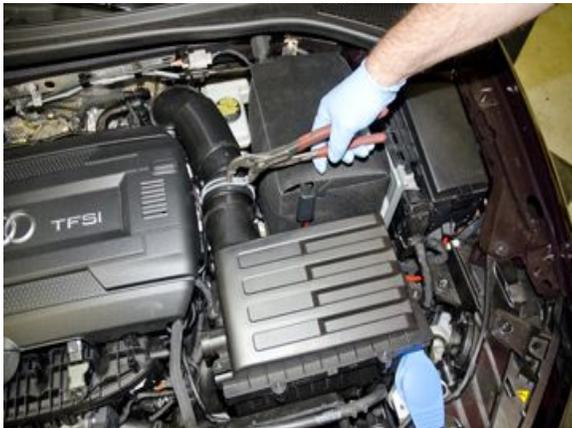
**4.** Using a 10mm socket, loosen and disconnect both battery cables – then remove battery cover. Using a 13mm socket, loosen and remove battery hold down. Remove battery.
