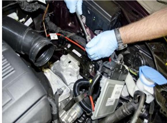
**9.** Using the 18mm socket remove the 3 bolts holding the transmission mount to the transmission. Once loosened remove the transmission mount from the car.
