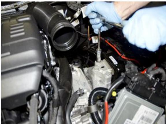
**10.** Installation of the pre-assembled transmission mount is the reverse of removal. torque values for the 18mm (3-M12) are 44ftlbs and for the 16mm (4-M10) are 34 ftlbs.
