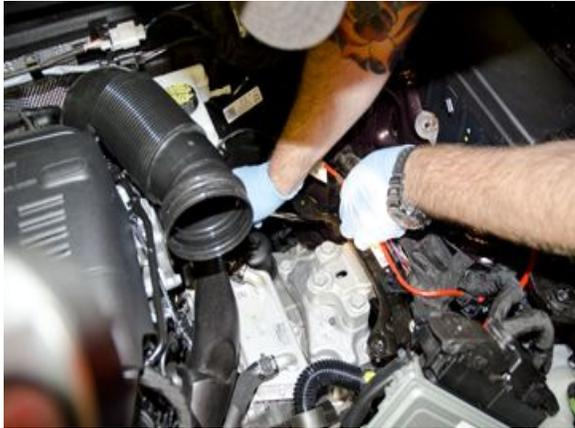
**8.** Using a 16mm socket, remove the four bolts that hold the transmission mount to the frame.
