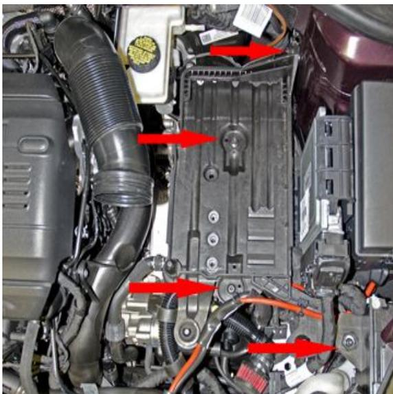
**6.** Once the battery tray is removed, unclip and pull aside the engine ECU. Using a 10mm socket remove the two nuts that hold the ECU cage to the fuse block, and remove the ECU cage.
