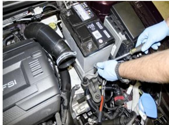
**5.** With the battery removed, locate the 4 10mm bolts and nuts that hold the battery tray in place. Remove all four and unclip the positive battery cable Harness. Pull out the battery tray.
